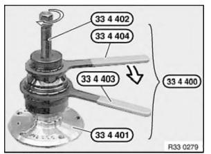
Compress special tool 33 4 401 with wrenches 33 4 403 and 33 4 404 until special tool can still just be turned in groove. Screw in special tool 33 4 402 . Detach inner bearing race.
